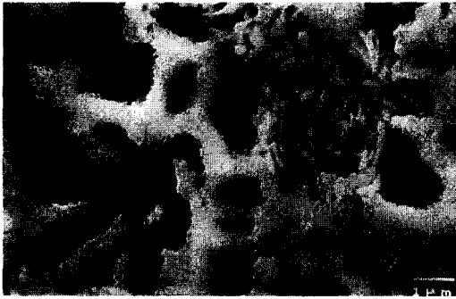
Fig. 5. Scanning electron image on U–10 wt% Mo fuel sample annealed at 400°C for 2000 h.
